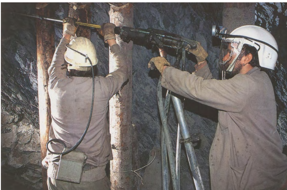
Introduction of the new Racal airstream system powered protective helmets against mercury vapours and silica dust in 1983. (Photo: B. Kladnik, Archive: CUDHg Idrija)
